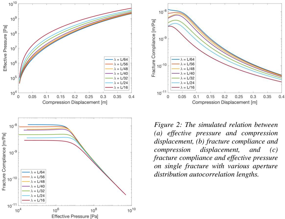
Figure 2: The simulated relation between (a) effective pressure and compression displacement, (b) fracture compliance and compression displacement, and (c) fracture compliance and effective pressure on single fracture with various aperture distribution autocorrelation lengths.
