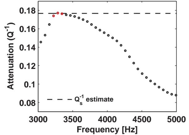
Figure 5: Field data example: estimate formation shear attenuation from dipole-flexural wave attenuation.
