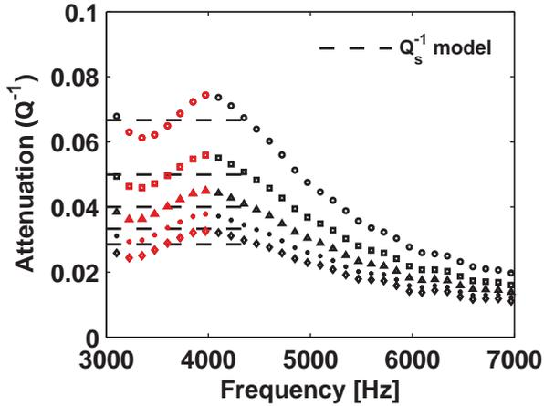
Figure 2: Synthetic data example: estimate formation shear attenuation from dipole-flexural wave attenuation. Different symbols denote different shear wave attenuation employed in the modeling.
