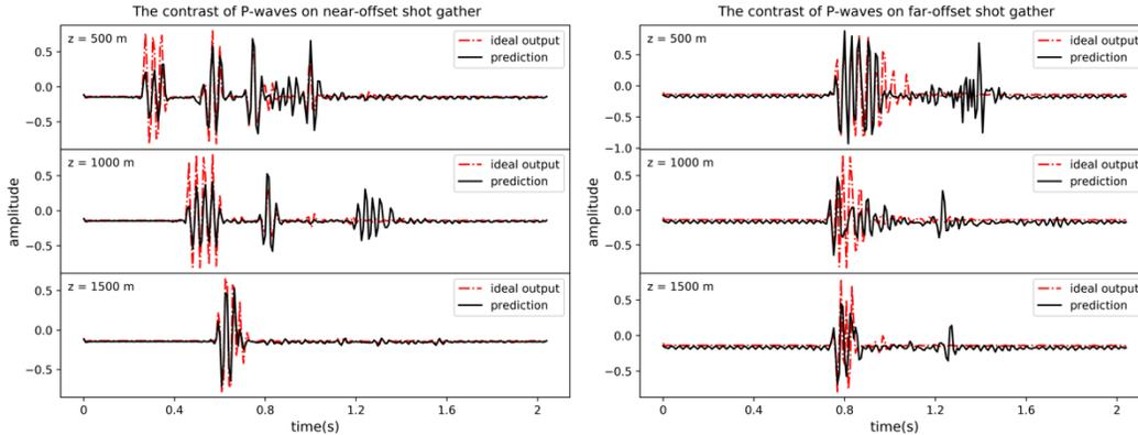
Figure 3: The signal contrast between P-waves extracted by divergence operator and GAN in the depth of  $z = 500\text{m}$ ,  $1000\text{m}$ ,  $1500\text{m}$ .
