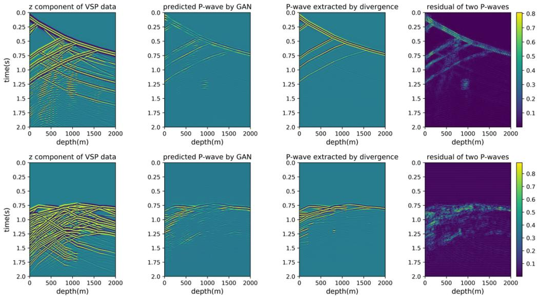
Figure 2: The results testing on synthetic data by GAN and contrast with the P-waves extracted by divergence operator.
