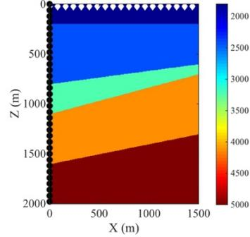
Figure 1: The P wave velocity (m/s) of a five-layered model and the distribution of the sources and receivers. Sources: white point near the surface; receivers: black point near  $x=0$ .
