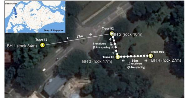
Figure 1. Site location and receivers’ layout plan.
