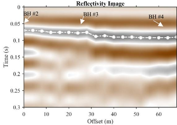
Figure 5. Image of estimated reflectivity at each trace, white dots are 1<sup>st</sup> peaks and connected by white dash line.
