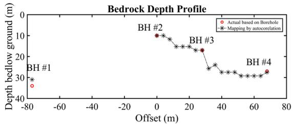
Figure 6. Estimated bedrock depth (black stars) with actual bedrock depth (red circles), and interpreted bedrock profile (dash line) from Trace #2 (BH#2) to Trace #19 (BH#4).
