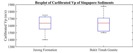
Figure 7. Boxplot show basic statistics of the average P-wave velocity of soil layers for the two major geology in Singapore.
