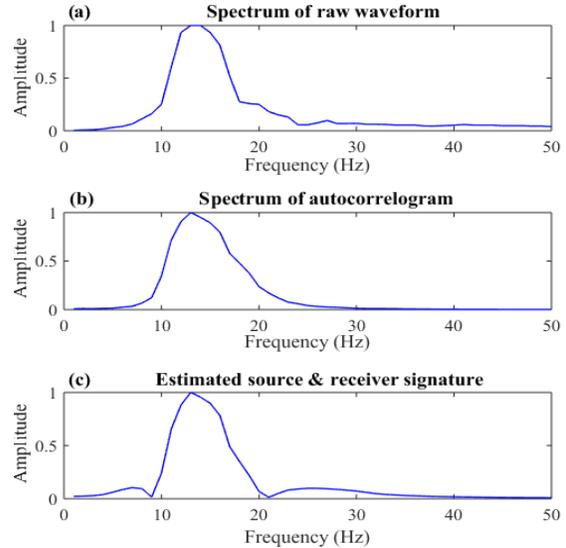
Figure 4. Normalized frequency spectrum at BH#3, from: (a) raw waveform, (b) autocorrelogram and (c) estimated source & receiver signature.
